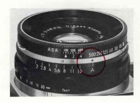
The Nikkorex Auto 35 incorporates an electric eye which automatically sets the aperture diaphragm for the correct exposure, depending upon the film speed and shutter speed. When using automatically, the red "A" on the aperture ring of the lens is alined with the black index dot.
