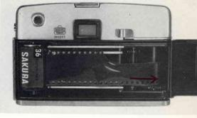
Push the rewind knob lock on the camera back to the left. The rewind knob will spring tp. Pull it up further by hand.
