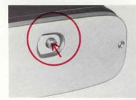
To rewind, first push in the rewind button found on the camera bottom. Then, push the rewind knob lock on the camera back to the left which allows the rewind knob to pop up. The rewind crank can be lifted up.
